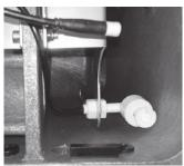
Push the connector through the opening and push it through the rubber plug. The small hole of the plug can be widened with a sharp knife to make this a
